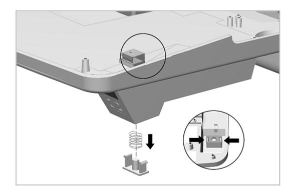
Figure 7-33. Removing the Monitor Support Cover Cap
